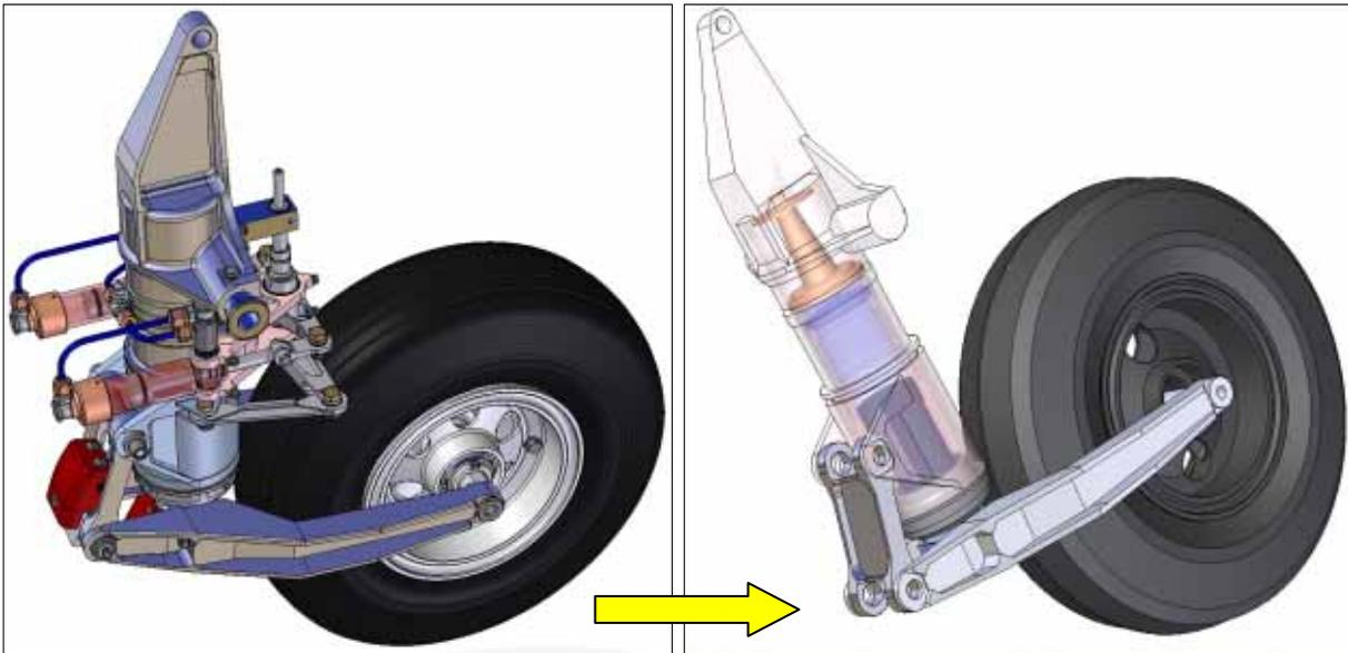
Fig. 3. The accurate MCAD model assembly simplification by non-important subassemblies deletion and replacing of important ones with simplified - geometry single parts
